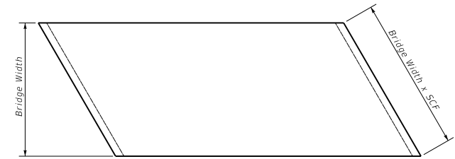
PLAN OF SUPERSTRUCTURE SLAB
